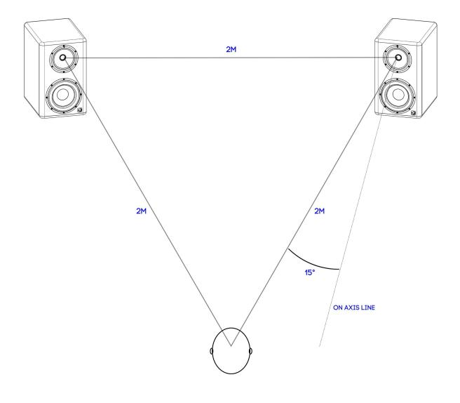
Having said this, Ganymede will retain its phase coherence and phantom center as close as 30cm away from the front of the cabinet. As a result, it can be worth experimenting with near-field listening positions that may help you mitigate the effects of poor room acoustics.
